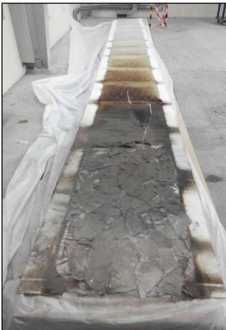
Photo 2: Specimen after the test (located near the fire end)
