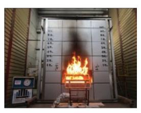
Test Specimen at 5 minute
