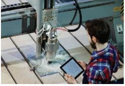
Drilling, countersink and milling of glass are carried out on modern high-precision CNC equipment which enables to create complex shapes and forms for individual orders.
