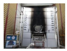
Test Specimen after 10 minutes at the end of fire test
