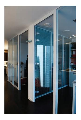
The construction of glass partitions in office space does not require much time and financial costs. As a rule, tempered glass is used in the manufacture. It is characterized by increased strength and durability against large loads. Various types of glass and processing technology are available. The use of matte and tinted decorative films is allowed.
